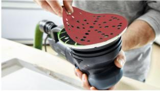
Quick changes Festool abrasives are changed without gluing or clamping, just pull one off and attach the next one.
