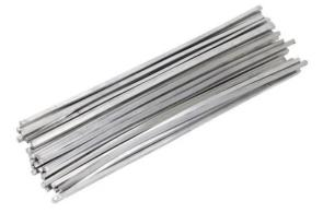
A lead/tin/zinc alloy which, when applied to a heated base metal, will melt & produce a strong corrosion resistant alloy coating. Used after welding on galvanised material resulting in a zinc coating equivalent to hot dip galvanise. **Features:**-Reapplies the Galvanised finish after welding Easy to apply
