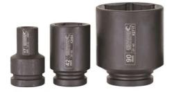
Kincrome Impact Sockets & Accessories are manufactured from Chrome Molybdenum Steel (Cr-Mo), hardened and tempered to perform in extreme conditions They are designed to be used with Pneumatic and Power tools where higher torque and force is required Kincrome Impact Sockets and Accessories meet and exceed the following international standards - ANSI, DIN 3121 & 3129
