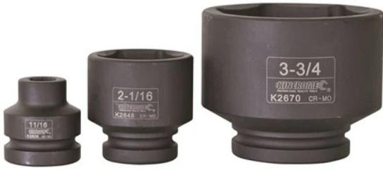
Kinchrome Impact Sockets & Accessories are manufactured from Chrome Molybdenum Steel (Cr-Mo), hardened and tempered to perform in extreme conditions. They are designed to be used with Pneumatic and Power tools where higher torque and force is required. Kinchrome Impact Sockets and Accessories meet and exceed the following international standards - ANSI, DIN 3121 & 3129.
