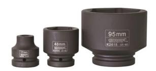
Kincrome Impact Sockets & Accessories are manufactured from Chrome Molybdenum Steel (Cr-Mo), hardened and tempered to perform in extreme conditions They are designed to be used with Pneumatic and Power tools where higher torque and force is required Kincrome Impact Sockets and Accessories meet and exceed the following international standards - ANSI, DIN 3121 & 3129
