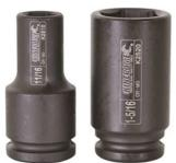
Kincrome Impact Sockets & Accessories are manufactured from Chrome Molybdenum Steel (Cr-Mo), hardened and tempered to perform in extreme conditions They are designed to be used with Pneumatic and Power tools where higher torque and force is required Kincrome Impact Sockets and Accessories meet and exceed the following international standards - ANSI, DIN 3121 & 3129
