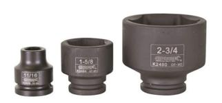
Kincrome Impact Sockets & Accessories are manufactured from Chrome Molybdenum Steel (Cr-Mo), hardened and tempered to perform in extreme conditions They are designed to be used with Pneumatic and Power tools where higher torque and force is required Kincrome Impact Sockets and Accessories meet and exceed the following international standards - ANSI, DIN 3121 & 3129
