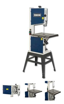
Offering woodworkers increased cutting capacity, power, and versatility at an entry-level price. 1HP motor drives the balanced cast-aluminium wheels at your choice of two speeds for standard cutting all types of woods, or for working with non-ferrous materials. A tilting table with two 'T' slots allows the use of a mitre gauge (available separately) or other cutting jigs on both sides of the blade. Includes steel stand. Rip fence with re-saw bar.
