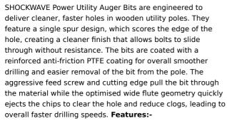
**Single Spur Design:** The single spur design scores the edge of the hole, creating a clean finish that allows bolts to slide through without resistance.
