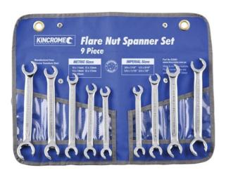
Forged from Chrome Vanadium Steel, hardened, tempered, chrome plated and polished for corrosion protection Designed for use on compression nuts fitted on petrol, diesel injection pipes and hydraulic gas or refrigeration systems, brake lines and hoses
