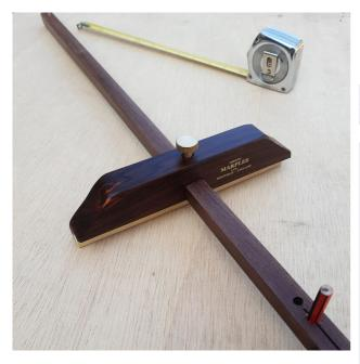
This **Panel Gauge** allows lines to be gauged past the centre of a 56" wide panel. The stem is approximately 30" long (this is based on the lengths of timber available at the time) and the head 9" wide with a brass wear strip fitted inside a rebate which rests on the edge of the panel to be gauged. One one end of the stem has a steel marking pin, the other end has the facility to insert a short, standard sized pencil to mark lines.
