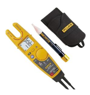
Measure voltage up to 1000V AC through the open fork, without test lead contact to live voltage, opening covers or removing wire nuts. Works with wires up to AWG 4/0 (120 mm<sup>2</sup>), carrying as much as 200A.
