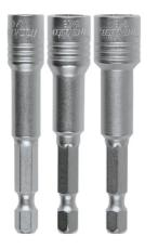
Impact XPS Magnetic Nutsetter is designed to drive hex head nuts and self-tapping screws in a variety of applications A hex shank allows for convenient use with high-torque impact drivers and driver-drills. Flat edges at the hex opening provides full contact with flanged hex head screws The magnet allows for easy one-handed operation
