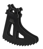
The AS200X GP Quick Switch Blades are used for general cutting of bricks and mortar. Ideal for chasing long runs of mortar as well as cutting openings into brick walls in a variety of building restoration and renovation projects. Also commonly used for toothing brickwork. **Depth:** 110mm (4 3/8")
