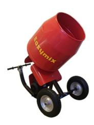
The T3EP mixer is available with either a petrol or electric motor. Built with a heavy-duty frame and bowl and uses Premium NSK bearings. Fitted with steel wheels and FLAT FREE Tyres (16 x 4.00-8). Comes standard with a fixed stand; the fatbowl and swivel stand are optional. Unloads at standard wheelbarrow height when on stand.
