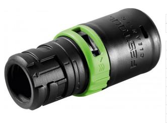
Hose connector for electric tool or suction nozzle|the bayonet fitting produces a secure connection between the mobile dust extractor and the power tool|with bypass for individually adjusting the air flow rate
