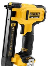
The DCN701 18V XR allows electrical contractors to secure cables on the jobsite faster and more consistently. The tool automatically adjusts depth of drive based on cable thickness and staple fits snuggly without pinching. A compact size of 200mm allows the user to work between joists and a built in LED light illuminates the working area when power isn't available.
