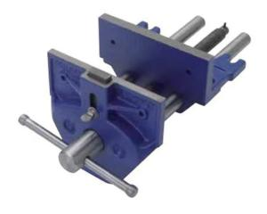
Plain screw mechanism works through a separate unbreakable nut housed beneath the body seating to ensure the constant alignment of the screw mechanism. Precision machined grey cast iron body and front to ensure a smooth, parallel action. Fitted with an adjustable front stop - or dog - that gives you additional clamping facility when used with a bench top, to provide a normal vice and a tail vice in one tool. To increase safety, the fused tommy bar will bend before
