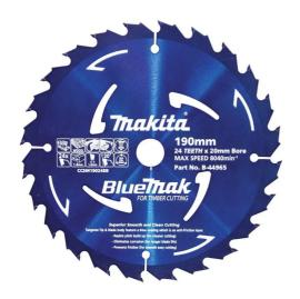
**MAKITA**® **BLUEMAK**® Circular Saw Blades feature a blue coating which resists "pitch" build-up and reduces friction during cutting. It also has an added advantage of eliminating corrosion.
