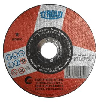
The BASIC\* cut-off wheel for stainless steel can be used to cut metal sheets, profiles, pipes, rods with small diameters and solid material. The chemical purity of this tool is a requirement of machining stainless steel in order to avoid impairments to the material, such as corrosion, pitting corrosion or a reduction in the fatigue strength. The 1.0 mm thick cut-off wheels are particularly suitable for quick, comfortable and low-burr cutting.
