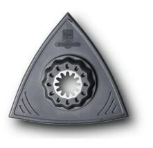
Thin, flat sanding pad for very narrow, flat openings (e.g. slats on cupboards, window shutters). Plastic carrier plate for preventing damage and marks on the workpiece. Triangular shape with hook and loop fastening. Pack of two.
