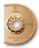
For cutting out damaged tile joints, slots in plaster, porous concrete and similar building materials and for cleaning and reworking deck joints. Not suited to very hard epoxy resin or cement joints. The economical alternative to diamond tools. Cutting width options approx. 1.2mm or 2.2mm Segmented, ideal for working in corners and on edges without overcutting
