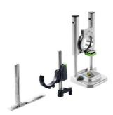
Allows exact positioning and sawing along a marking, as well as plunge cuts to a specific depth; position guide; depth stop; adapter for tool free attachment of AH and TA Max. plunge depth with depth stop 56 mm; Max. plunge depth with sliding shoe 20 mm; Max. plunge depth with position guide 60 mm; Depth setting with adjustments 1.5 mm; Weight 0.47 kg
