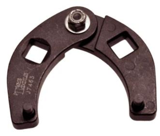
Fully adjustable to fit hydraulic cylinders on vehicles and machinery having gland nuts with pin holes located on the face of the gland nut or fitting. Works on both 7/32" and 1/4" (5.5 or 6.4mm) pin holes.
