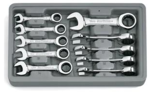
72 tooth ratcheting box end needs a minimal 5  $^\circ$  to move fasteners vs. 30  $^\circ$  for standard wrenches
