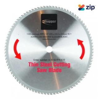
The Slugger metal saw blades are designed for fast and accurate cuts in mild & thin metal, aluminium and stainless steel. Compared to traditional abrasive-type blades, Slugger metal blades perform faster, more accurate cuts and maintain a lower temperature with less dust. Thin Steel up to 1/4 in (6 mm) solid material. Fits:-MCC14 14" Slugger Metal Cutting Saw
