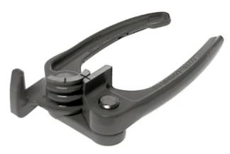
Three sizes in one, for accurately bending small diameter annealed copper, aluminium and thin wall steel tubing. Angle settings are marked on tool for accuracy of bend and repetitive bending capability. Strong durable die cast aluminium construction. **Specifications:**
