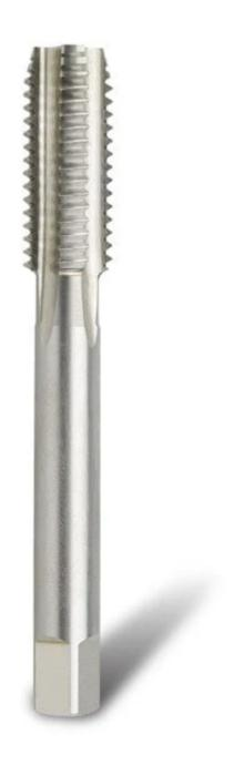
5/8" x 24 UNEF Bottoming HSS Tap HSS UNEF Bottoming Hand and Machine Tap. Unified National Extra Fine is a subset of UNF in which the thread forms feature a greater number of TPI than the standard UNF series.
