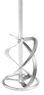
Helical stirrer with 2 spirals for chuck with clamping range equal to or greater than 10 mm. For thorough mixing of viscous substances, adhesives, filling compounds and ready mixed plasters. For mixing volumes of 30 kg - 60 kg.
