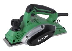
Features: Lightweight and compact Heavy-duty aluminium housing Maximum rebating depth of 9mm Able to be connected to dust extraction equipment Blade protection stand to protect the blade from catching when placing the tool down **Specifications:** Input Power: 620W No Load Speed: 17,000rpm Blade Type: 82mm Max Cutting Width: 82mm Max Cutting Depth: 2.6mm Length: 296mm
