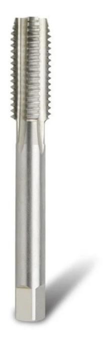
HSS Metric Fine Bottoming Hand and Machine Tap. Metric Fine angle of thread is 60 degrees. The crest is flat and the thread has clearance at the root allowing external thread and internal thread to engage well. Larger root radius and lower thread height enable easy screw thread processing and increase thread screw strength. The major diameter of external thread and pitch are specified by a simple numerical value (most commonly measured in millimetres).
