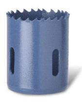
**35mm Bi-Metal Hole Saw 7010-35 by Bordo** Bordo bimetal hole saws are premium quality, general purpose saws suitable for a wide variety of materials and applications. The high-speed steel cobalt (HSS-Co) cutting edge provides shock resistant teeth and resists tooth strippage. 4/6 positive tooth configuration allows for fast, smooth cuts and less vibration.
