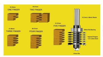
Produces a beautiful, strong exposed finger joint on end and long grain. Make central identical cuts on both pieces always using the butting edge cutter, invert one piece & fit together (see Insert Two Finger picture). **Features:-**
