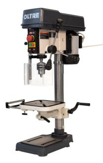
This is a slightly larger bench pillar drill for hobby use. Robustly made from cast iron and machined steel for stability and strength. It has a true running chuck spindle and a good fit of the quill assembly into the headstock casting to ensure consistent drilling. Powered by a 1/3HP induction motor, Variable speed is adjusted with one simple lever and the speed is displayed on a large digital read-out. **Features**
