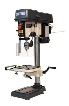
This is a slightly larger bench pillar drill for hobby use. Robustly made from cast iron and machined steel for stability and strength. It has a true running chuck spindle and a good fit of the quill assembly into the headstock casting to ensure consistent drilling. Powered by a 1/3HP induction motor, Variable speed is adjusted with one simple lever and the speed is displayed on a large digital read-out.
