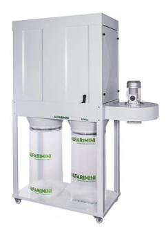
Euro 2 is a professional extraction unit with specific features in the Euro range by Alfarimini. It therefore features sturdy painted sheet metal and faired and wheeled frame. Its three-phase motor has 4 HP power and is always supplied with a 1.5 m supply cable and motor protection circuit breaker. The standard version includes 18 cotton filter sleeves, an ideal fabric for filtering coarse dust and wood shavings, plastic and others.
