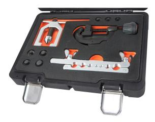
SAE Double Flaring Tool Kit Holds pipe sizes: 3/16, 1/4, 5/16, 3/8, 7/16, 1/2 & 5/8" Aluminium alloy casting tube cutter from 3-30mm Steel casing, yoke & screen bar 7pc adaptor Stored in blow mould case
