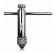
Designed to give reach and leverage required for accurate tapping. Jaws conform to tool being held making it rigid and less prone to becoming loose. Sliding handle enables work in tight spaces. Ratchet can be set for right or left hand operations or direct engagement in neutral position. Self centering hardened steel jaws Knurled chuck sleeve. Holds all hand turned tools
