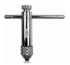
Designed to give reach and leverage required for accurate tapping. Jaws conform to tool being held making it rigid and less prone to becoming loose. Sliding handle enables work in tight spaces. Ratchet can be set for right or left hand operations or direct engagement in neutral position. Self centering hardened steel jaws Knurled chuck sleeve. Holds all hand turned tools
