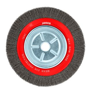
Josco Wheel Brushes with crimped wire are suitable for bench grinders. Crimped wire construction allows for softer brushing and light paint and rust removal.
