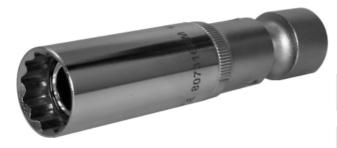
3/8" Drive ball type universal spark plug socket with a permanent magnet. Ball type universal joint and thin wall socket is required when installing or retrieving from the spark plug hole.
