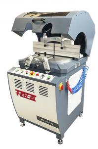
FN 420AC Automatic Up-Cutting Saw Machine is used for straight and angular cutting operations of aluminum, wooden and plastic materials. The machine can be used the lateral cutting mode and longitudinal cutting mode.
