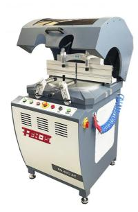
FN 420AC Automatic Up-Cutting Saw Machine is used for straight and angular cutting operations of aluminum, wooden and plastic materials. The machine can be used the lateral cutting mode and longitudinal cutting mode.
