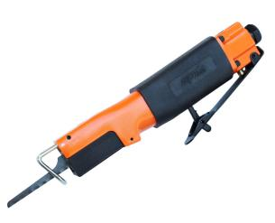
Free Speed: 10,000 Strokes per min. Capacity: 1.6mm Length: 235mm Air Consumption: 108L/min Average\* Front Exhaust Ideal for the automotive industry
