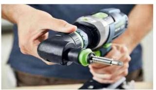
Practical attachments with quick angle adjustment Very quick angle adjustment simply by rotating the green ring. The attachment no longer needs to be released from the machine. Even the eccentric adapter for screwdriving close to edges is equipped with quick angle adjustment.
