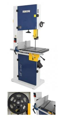
10-342 is an entry level machine to this larger capacity category. 2HP motor provides plenty of power behind the single 10.5m /min. blade speed of the machine. Cast iron table includes a single 'T' Slot for use with Miter Gauges or other cutting jigs. This powerful bandsaw is outstanding value and a more than capable addition to any workshop.
