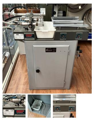
Semi automatic glue spreader with twin heads with many accessories for dovetail glue spreading or also cabinet and kitchen door application.
