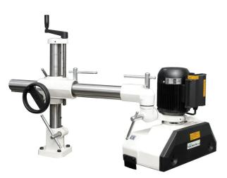
This Automatic Power Feeder is ideal for pushing large material/stock through a Router Table, Spindle Moulder, Saw, Planer / Thicknesser, and other Machinery.
