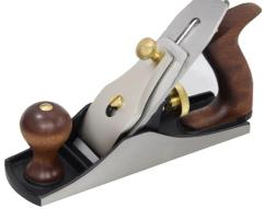
As the name suggests a very good plane for general smoothing and final finishing work. A must for every workshop. The sole of the plane is available in a plane finish as well as a ribbed finish for a smoother action on damp or resiny lumber. The long sole of the planes ensure good results for flattening large surfaces without any bumps and valleys. The planes have a ductile cast iron body which is fully stress relived and carbon steel blades.
