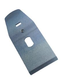
The Clifton 440 Cap Iron is a single piece design, made from vacuum toughened and hardened 01 steel and has an approximate thickness of 3.6mm. The cap iron is designed to sit on the plane blade to help prevent tear out and also to reduce vibration in the blade which in turn can cause chatter. This will offer a great way to reinforce your blade and ensure you get the ultimate performance from your plane blade. Pairs well with our 01 cryogenically treated plane blades.
