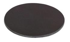
The 150 mm diameter StickFix Platin 2 sanding discs are an ideal abrasive for super fine finish on fillers, finish coats, solid surface, fibreglass and plastics. Platin 2 sanding discs range from S400 up to S4000 grit abrasives for extra fine sanding. A foam backed, silicon carbide based abrasive with a stearate coating specially developed for high gloss finishes on closed surface materials. StickFix hook and loop design for quick and efficient abrasive changes.
